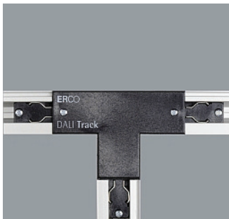
79228.000 DALI T-connector Polymer. Earth conductor, right. Feeding possible. Through-wiring. Black CE
