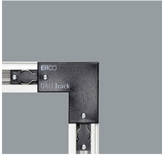
79227.000 DALI L-connector Polymer. Earth conductor outside. Feeding possible. Through-wiring. Black CE
