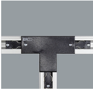
79329.000 3-circuit T-connector Polymer. Earth conductor, left. Feeding possible. Through-wiring. Black 🔌 ⚡ CE
