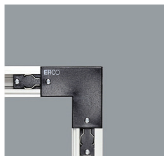
79326.000 3-circuit L-connector Polymer. Earth conductor inside. Feeding possible. Through-wiring. Black
