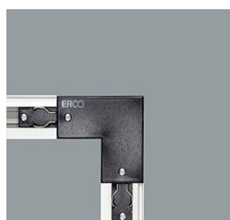
79327.000 3-circuit L-connector Polymer. Earth conductor outside. Feeding possible. Through-wiring. Black
